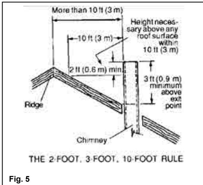
Limit connector pipe to 8 ft. or less, with no more than two elbows. All horizontal sections should have 1/4 in. rise per foot. The chimney must be capable of providing a draft reading of at least .06 in. of water column. A barometric damper can be installed to prevent excessive and erratic draft. All connector pipe should be secured with sheet metal screws at each joint.
